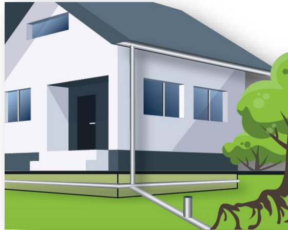
ILLEGAL ROOF CONNECTIONS
