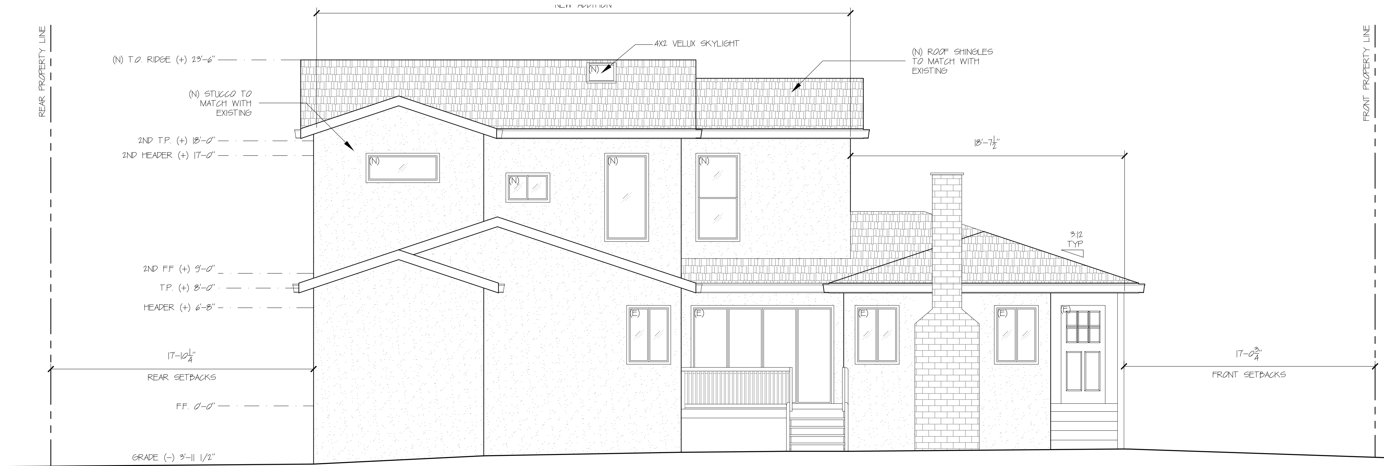
1 PROPOSED LEFT SIDE ELEVATION (NORTH) SCALE = 1/4" = 1'-0"
