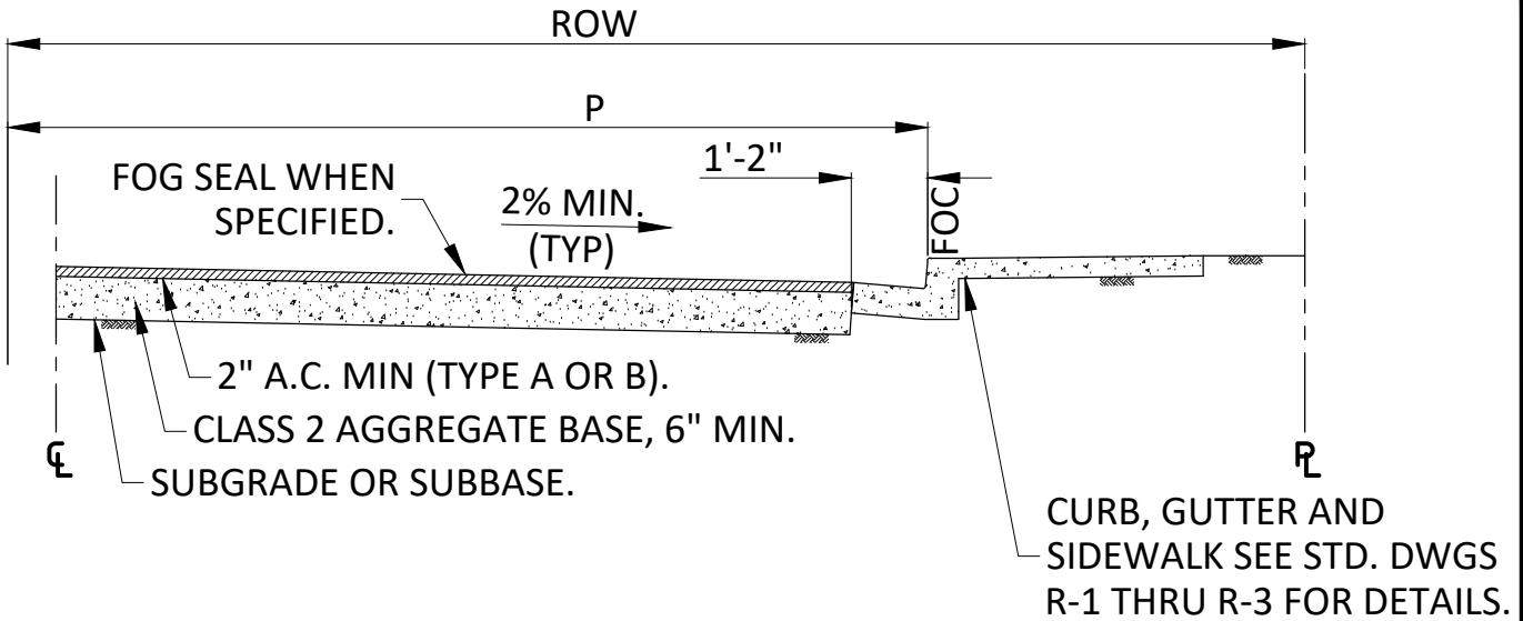
NOTE: ALL MATERIALS IN THE STREET SECTION SHALL HAVE A 95% MINIMUM RELATIVE DENSITY OF COMPACTION.
