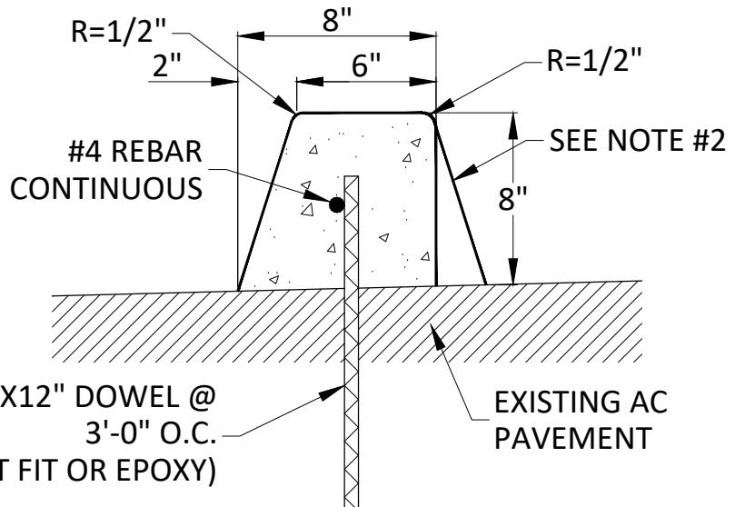
NOTE: DELETE #4 BAR & DOWEL IF CURB IS EXTRUDED. FOR EXTRUDED CURB CONSTRUCTION, EPOXY RESIN ADHESIVE SHALL BE APPLIED IN LIEU OF BAR & DOWEL REINFORCING.
